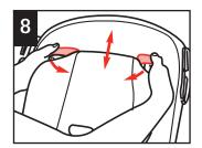
Rotate headrest/harness adjusting levers in. Move headrest up or down to adjust. Make sure headrest is locked into place. **NOTE:** The highest position is for beltpositioning use only.
